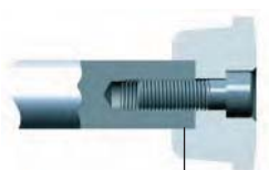
Press fit (screw loctited for security).
